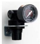
**Monnier** has donated the secondary regulator, which has a yellow ring around it. This is also a relieving regulator. Its purpose is to allow you to have a reduced pressure leg, if needed. There is an arrow denoting the direction of flow. The gauge may be placed in either of the other ports. The Monnier bag provides you with plugs to put into the gauge ports.
