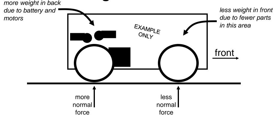
The weight of the robot is <u>not</u> equally distributed among all the contacts with the floor. <u>Weight distribution</u> is dependent on where the parts are in the robot. This affects the normal force at each wheel.
