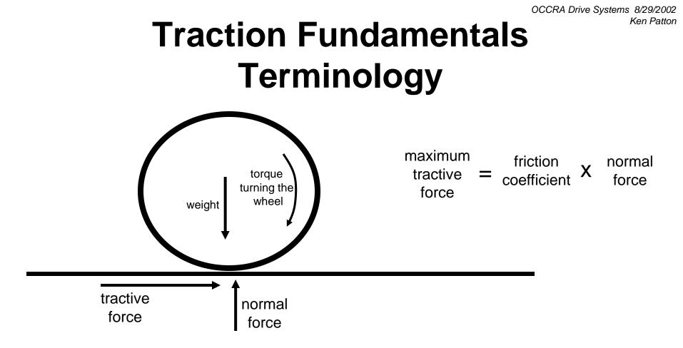
The <u>friction coefficient</u> for any given contact with the floor, multiplied by the <u>normal force</u>, equals the maximum <u>tractive force</u> can be applied at the contact area.
