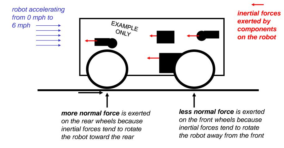
In an extreme case (with rear wheel drive), you pull a wheelie In a really extreme case (with rear wheel drive), you tip over!
