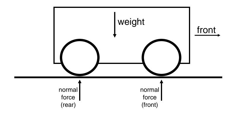
The <u>normal force</u> is the force that the wheels exert on the floor, and is equal and opposite to the force the floor exerts on the wheels. In the simplest case, this is dependent on the weight of the robot. The normal force is divided among the robot features in contact with the ground.
