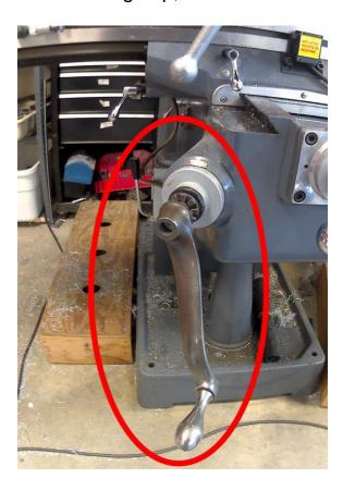
This crank controls the position (Z) of the bed. Clockwise makes bed move away, counter-clockwise makes the bed move towards you.
