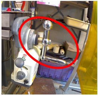
This crank controls the (X) position of the bed automatically, and the button makes the bed move faster automatically.
