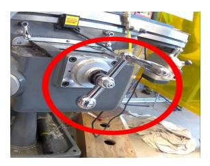
These cranks controls the position (X) of the bed manually. Direction depends on the side.
