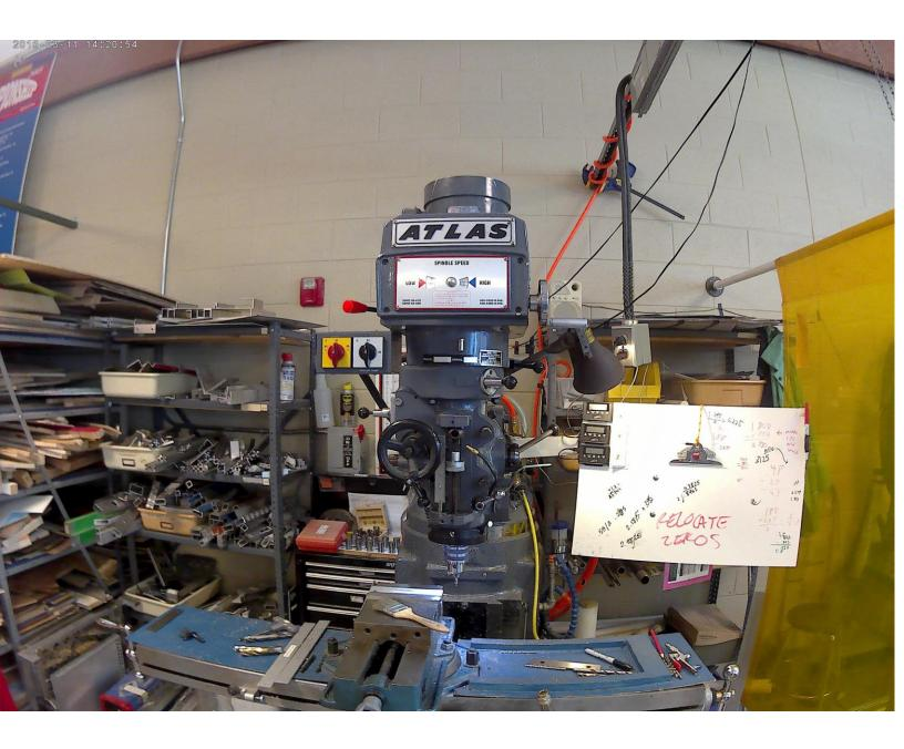
The Atlas vertical mill shares some similarities with the drill press, yet the mill is more precise, more powerful, and more dangerous if you're not careful. Unlike the drill press, the mill has a moving bed that moves on XYZ axises, unlike the drill press, which has a stationary bed and a moving chuck.
